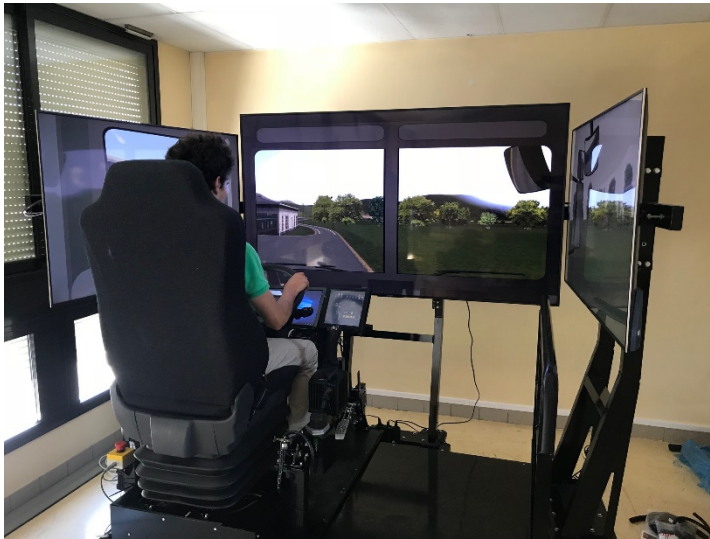
SYM2B Truck Simulator with 6 axis Motion chair
