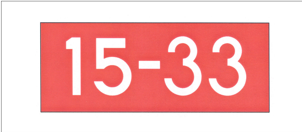
FIG 2-3-24 Runway Holding Position Sign
