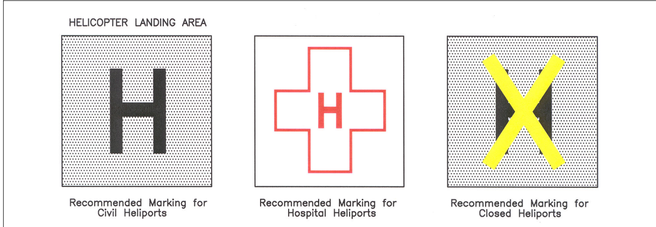
FIG 2-3-23 Helicopter Landing Areas
