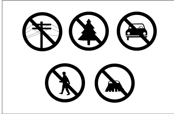
FIG 10-2-5 Landing Zone Hazards
