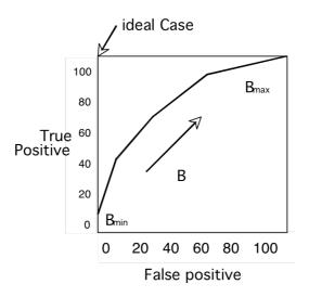
the ROC plots the True Positive Rate (TPR) against False Positive Rate (FPR) for a classifier as a function of the global bias B.
