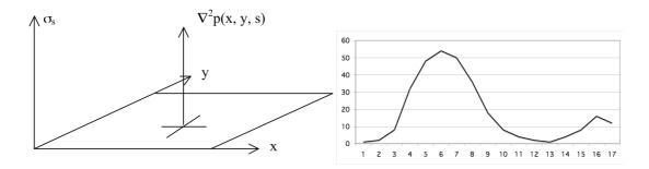
A change in viewing distance at x, y shifts the function  $\nabla^2 p(x,y,s)$  in s. The function remains the same. Thus the maximum is a local invariant.
