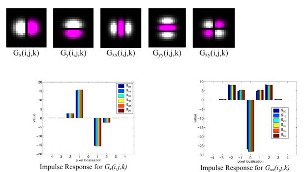
Impulse response for Gaussian derivatives for pyramid levels k=0,1,2,3,4,5.
