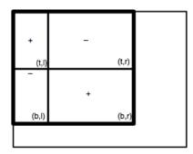
Notice that this is equivalent to a product of the image with a rectangular window with constant coefficients of size M, N:  $W_{m,n}(i,j)$ .
