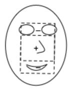
Some features respond to the appearance of a face. These can be used to determine if the imagette contains a face or not.
