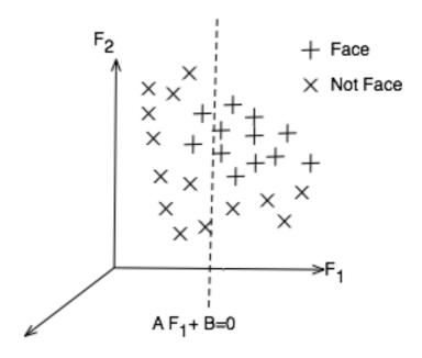
Each feature can be used to define a hyper-plane  $\langle W, H_n \rangle + b = 0$ .
