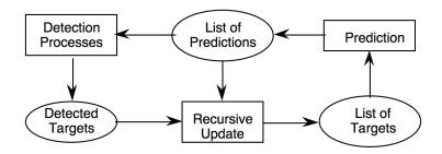
Detection can be provided by detecting the blob using color statistics within a target "Region of Interest" given by a bounding box centered on a previous position. The size of this box is determined by the estimated size of the blob enlarged by the uncertainty P.
