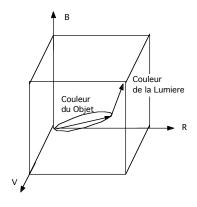
Suppose the image contains only a single (non-planar) object that obeys a bi-chromatic reflection model. If the image contains a specular reflection, then two clear axes will emerge.
