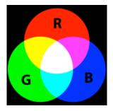
The RGB model "pretends" that Red, Green and Blue are orthogonal (independent) axes of a Cartesian space.
