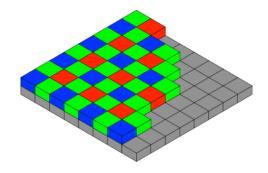
The voltage values on each sensel are converted to numeric values, interpolated and processed to provide image pixels. This step is sometimes called "image reconstruction" in the image processing community, and is generally carried out on the retina. The result is generally an image with colors coded as independent components: RGB.
