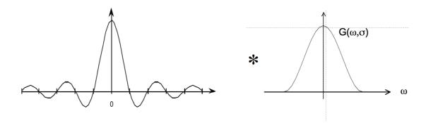
For N < 7, the ripples in WN(w) dominate the spectrum and corrupt the resulting Gaussian.
