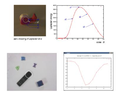
The scale of the maximal Laplacian is an invariant at ALL image points.
