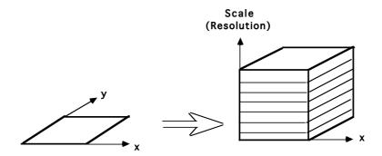
Scale space represents a 2D image in a 3D space, where the 3rd dimension is "resolution" or scale. This can be used to make image descriptions invariant to changes in size.
