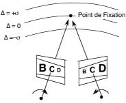
Eye movements can decomposed into "Version" and "Vergence". Version perceives relative direction in head centered coordinates. Vergence perceives relative depth.
