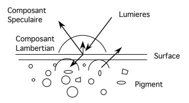
Most reflectance functions can be modeled as a weighted sum of two components: A Lambertian component and a specular component.
